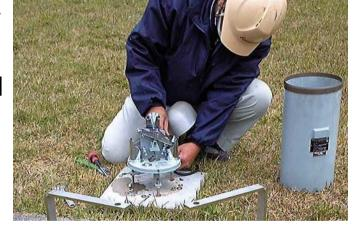
Rain gauge overhaul in Meteorological Instrument Center every 5 years.
